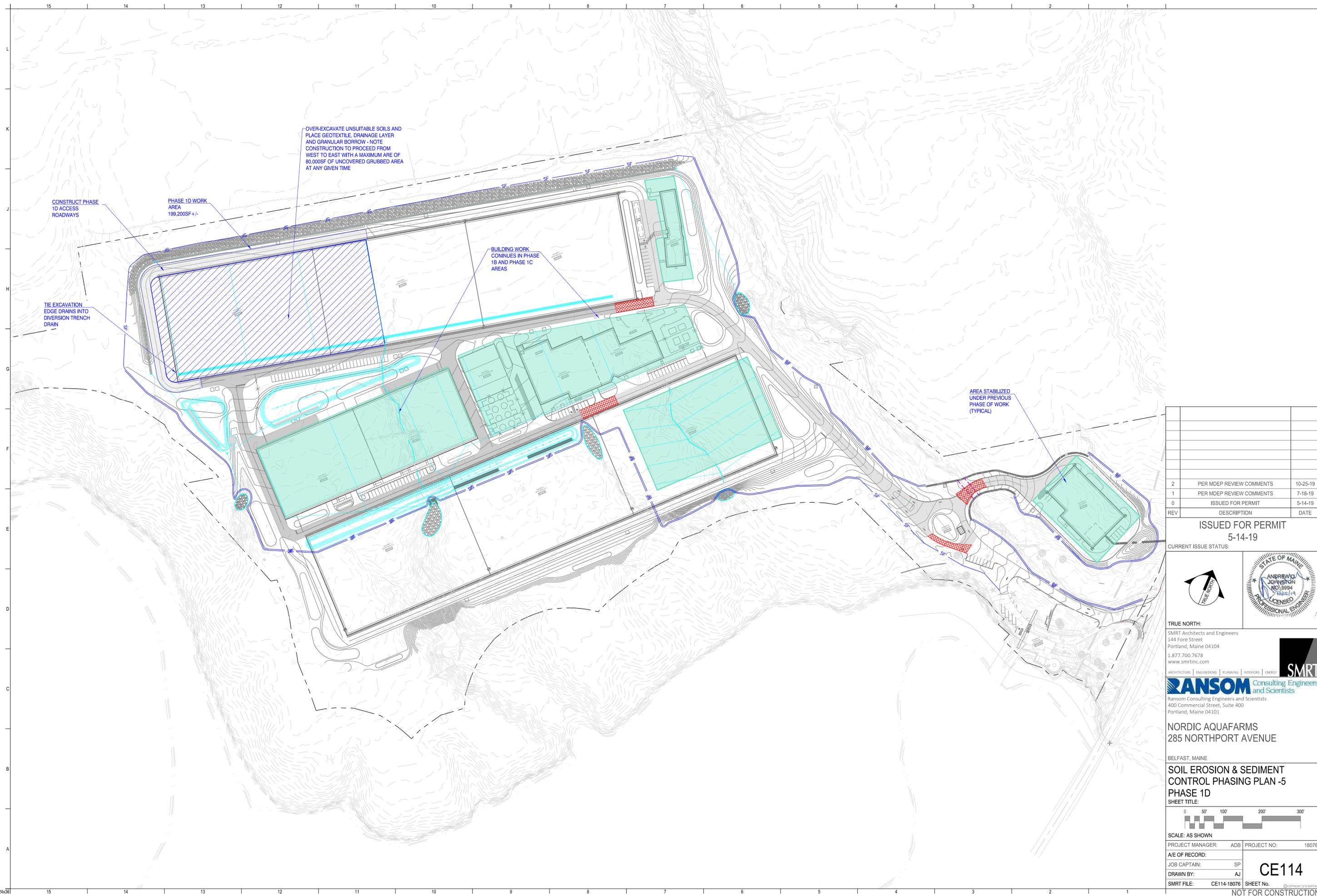
OVER-EXCAVATE UNSUITABLE SOILS AND PLACE GEOTEXTILE, DRAINAGE LAYER AND GRANULAR BORROW - NOTE CONSTRUCTION TO PROCEED FROM WEST TO EAST WITH A MAXIMUM ARE OF 80,000SF OF UNCOVERED GRUBBED AREA AT ANY GIVEN TIME
