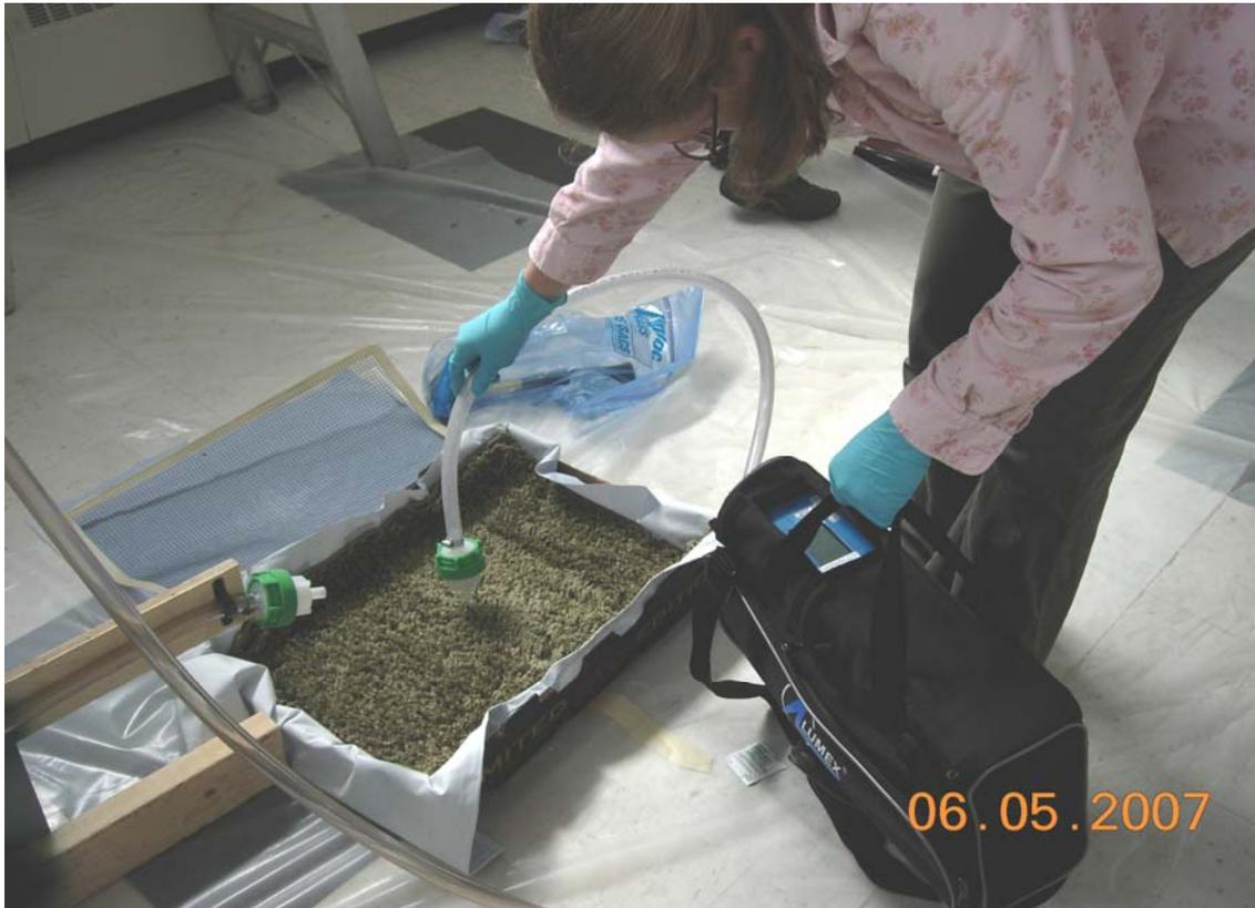
Figure B-3. Taking near-surface mercury measurements.
