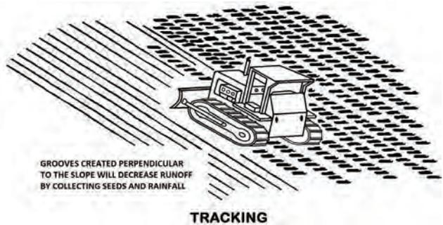
**GROOVING** is the process of using agricultural equipment such as a tiller (plow, chisel) or disc harrow across the slope, leaving small ridges. The grooves should be less than 15 inches apart and less than 6 inches deep. Grooving should be limited to slopes flatter than 3:1.
