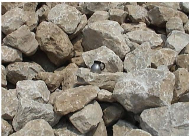
sizes that will provide a cohesive, strong and well blended cover with minimum voids. The desired distribution of stones may be obtained by selective hand placing.
