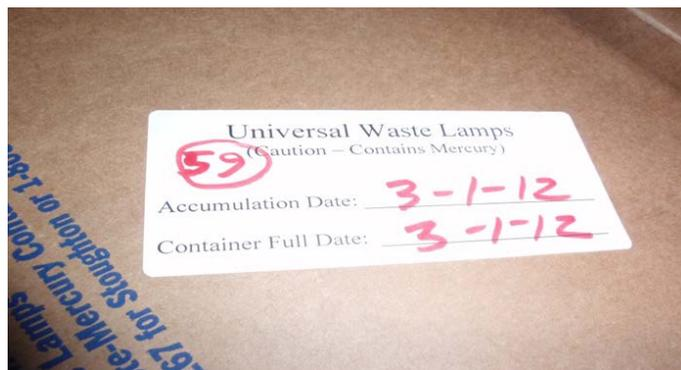
6. Universal wastes cannot be stored for more than **365** days from the date the waste is *first placed* in the container. However, there is an exception, which allows additional storage time where it is needed to fill a container of waste no larger than the following container sizes and the container is shipped **no more than 90 days** from the date the container is filled\*:
