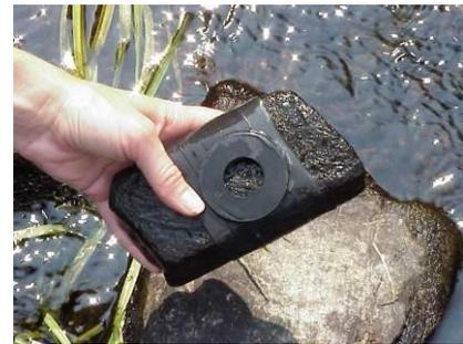
**Figure 8. Wrapping sampling device around cobble**
