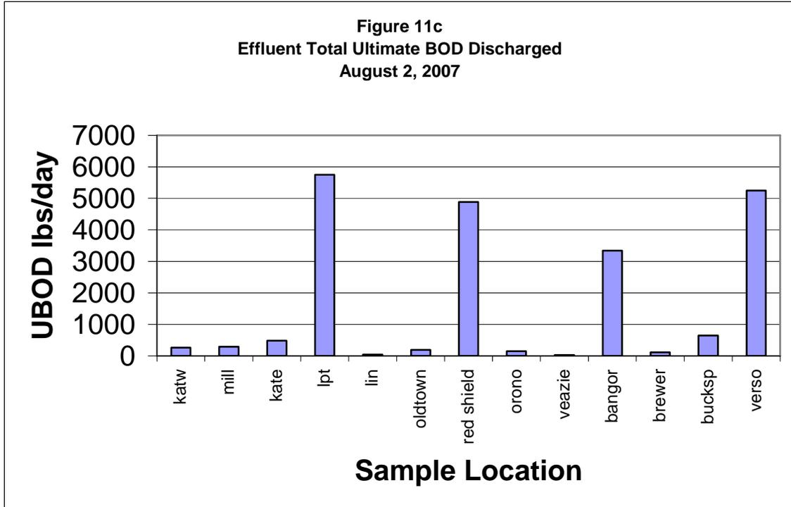
It can be seen that, although Bucksport has a much higher waste strength when compared to other discharges, its low flow volume results in a small pollutant load. The higher waste strength is expected since this town has primary treatment compared to secondary treatment of the other discharges. Many of the discharges sampled during the survey had very low concentrations of BOD, indicating good treatment.
