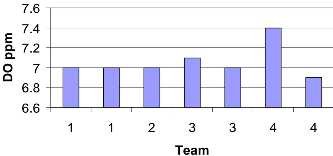
Field duplicate samples were collected for all parameters at a river, estuary, tributary, and effluent station each day during the intensive survey. When the results for some of various parameters are compared graphically for ambient (Figures 18-28) and effluent (Figure 29-30) samples, good agreement occurs for most of the samples. An examination of the deviation of the duplicate from the actual sample indicates the following:
