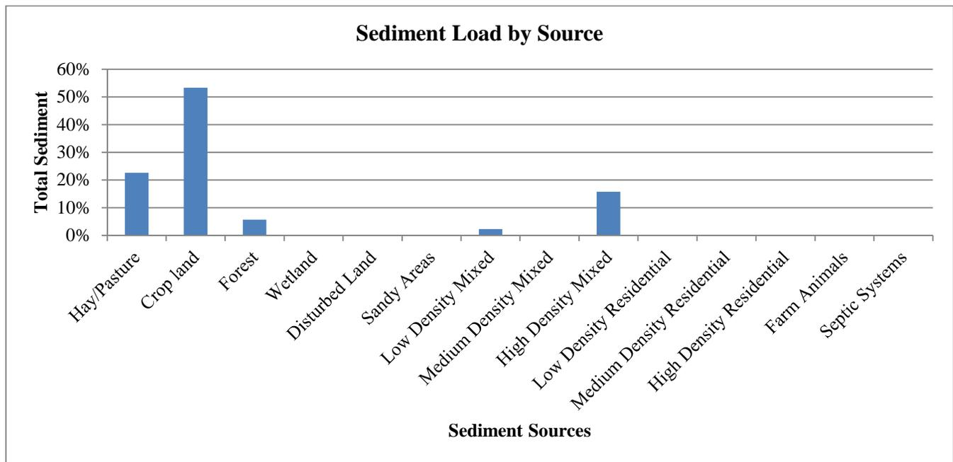
**Figure 5: Total Sediment Loads by Source in the Mill Stream Watershed**
