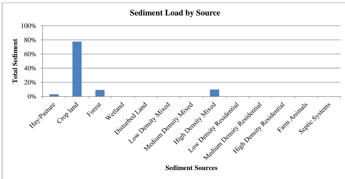
**Figure 4: Total Sediment Loads by Source in the Burnham Brook Watershed**
